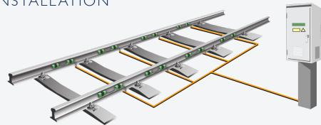
Our patented bolt-on sensors do not require the track to be closed during installation and maintenance which dramatically reduces traffic interferences.
